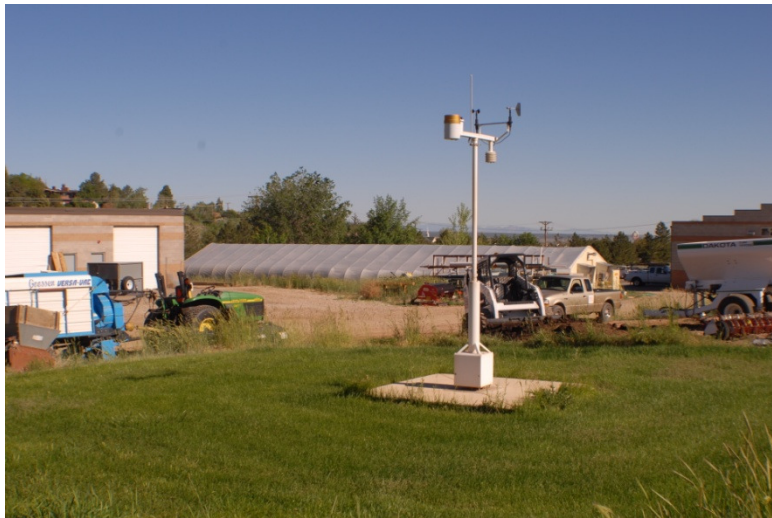
On the Southern Utah University campus the Maxicom weather station provides the irrigation system with data to turn the sprinklers on or off
